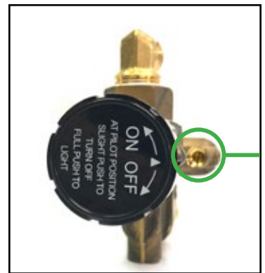
Fig. 13 - SPV Option 1 with Adj. Screw (in 3 o'clock 'PILOT' position)
